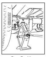
3. Position the jack under the vehicle as shown.
